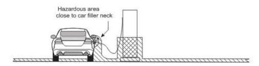
REFUELLING: EXTENT OF HAZARDOUS AREA DEPENDENT UPON VEHICLE POSITION, WHETHER FUEL IS PETROL OR DIESEL, AND WHETHER VAPOUR RECOVERY IS INSTALLED
